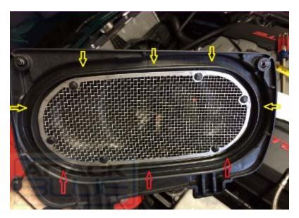
**STEP 7:** Install the attack Blue Filter into the factory air cleaner housing.
