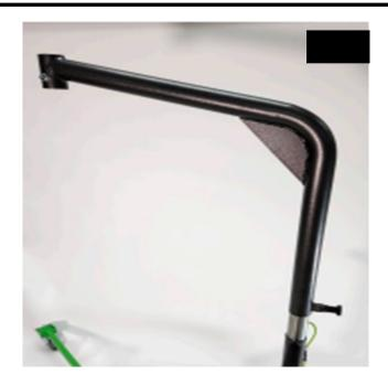
Remove the Crossbar: Remove the Locking Pins and Locking Knob (fig 9) to release the Crossbar, then slide the Crossbar off the lift. Be sure to pull the Green Cable while removing the Crossbar to be sure it doesn't get stuck.
