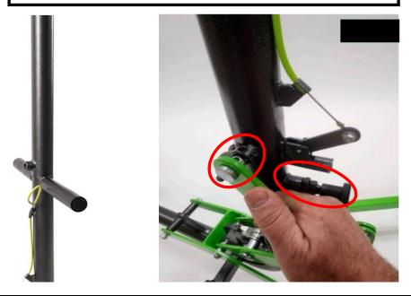
Remove the Bearing Post: Remove the two securing bolts, then remove the Bearing Post (NOTE: the Bearing Post will be exposed after the Crossbar has been removed)
