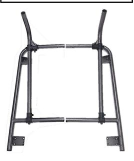
3.) The next step is to grab the two **8in Aluminum Insert (Long)** and four **M10x50 Bolts/Nuts**. Install the 8in Inserts (x2) into the Left or right half of the base with two M10x50 Bolt/Nut **(Use the 17mm wrench & 8mm Allen Key)**. After installing the 8in Inserts in one half of the base, you will then take the other half, slide it on, and then tighten it together with the other two M10x50 Bolts/Nuts.
