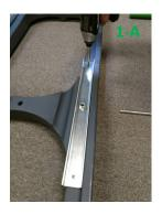
2. Un screw C-Channel, save screws (1-A). Going to install C-Channel cross member as shown. Press down after lining up center hole on Base (1-B).
