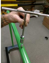
6. Install green Handle into base with Center Rod going through center (place the nut on the end of the Center Rod once through the Green Handle)(2-A) *Twist with your fingers to thread the Center Rod into the Base (2-B)*. Then tighten the nuts on Handle end. (THE CENTER ROD WILL ADJUST YOUR DOOR WEIGHT PULL-ING THE CENTER OF THE BASE UP WHEN YOU FIRST PLACE YOUR DOORS ON BY TURNING THE NUTS ATOP THE HANDLE AS SHOWN.
