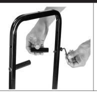
With the RocknRoller Multi-Cart extended and both handles raised, install the round support tubes. Insert the 5/16" low profile socket head screws into the handle's predrilled holes from the outer edge, so the support tube in inside the handle. Make sure each tube is set to the same height before screwing them in securely.
