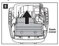
➤ Remove the foam cover to expose the evaporator coil and control board wiring.
