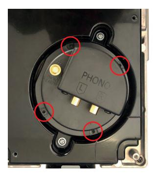
Now remove the socket so you can have access to the wires
