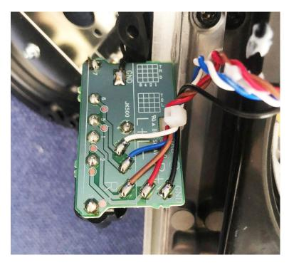
Note: you can unscrew the 2 screws on the external portion of RCA socket to have better access to pcb and cables.
