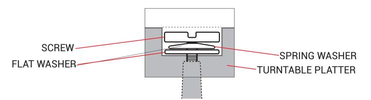
Carefully remove the turntable platter with two fingers and place it on a soft surface
