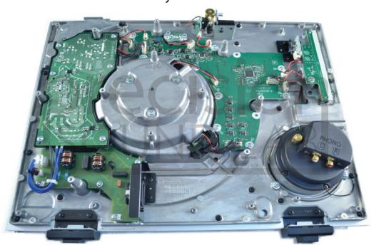
Unhook the two blue cables and the black one from the cable tie
