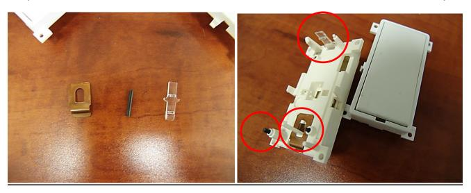
2. Align the plastic-set to the heat-sink, insert one of the side lock-tab first, and then press in the other side for attachment.
