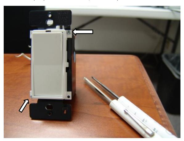
2. The plastic-set is attached to 4 places: <u>2 tabs</u> locked to the circuit board (top and bottom) and <u>2 side</u> <u>tabs</u> attached to heat-sink.
