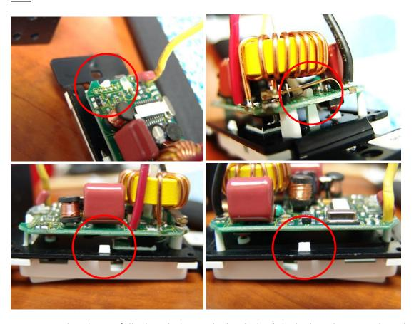
3. Using your thumb, carefully detach the top lock-tab that's locked on the circuit board.
