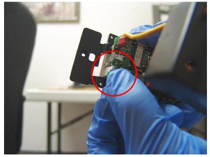
4. Once the top lock-tab is detached, the bottom lock-tab is still attached. Use your hand to grip the circuit board; the other hand grips the heat-sink, slighting twist to left to unlock the lower lock-tab. There will be a slight click sound. Be careful not to twist too much to cause the triac legs to break.
