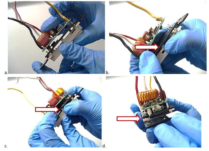
3. Grip the unit securely, using the flat-head screw driver, slightly pry to stretch the top lock-tab outward a little, press the circuit board down so the lock tab will lock onto it. Make sure the small plastic leg aligns with the tiny hole of the circuit board (circled below)
