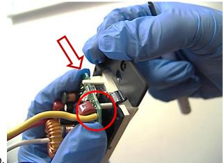
4. At the bottom side, the bottom lock-tab is probably sitting 80% through the hole (arrow pointed in picture a). Align the circular tubing of the plastic-set with the hole on the circuit board (circled below in picture a). Utilize the flat-head screw driver to press onto the circuit board (right under the toroidal inductor) while your thumb presses against the plastic-set to lock everything tight (see picture b and c below)
