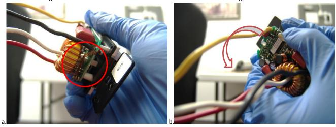
5. Once you notice lower lock-tab is detached from the circuit board, use your thumb to detach (press in) one of the side lock-tabs that clips to the heat-sink.
