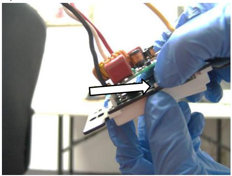
7. The plastic-set is now off. Remove the <u>light pipe</u>, <u>metal clip</u>, and <u>black plastic rod</u>.
