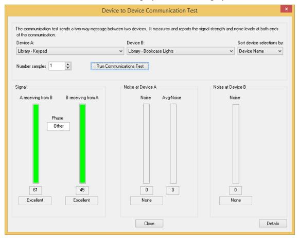
This is a very simple test to use. Just select two devices and press the *Run Communications Test* button. Device A sends a command to Device B and Device B responds. UPStart listens in on that conversation and reports the signal and noise levels at both ends of the conversation.
