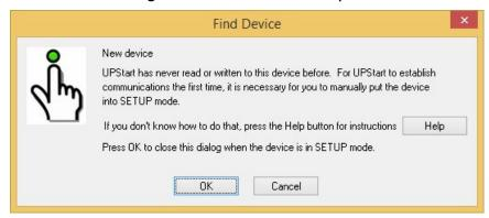
After the device is in the Setup Mode press the OK button. UPStart then performs the command steps necessary to read the device's configuration memory.
