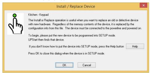
As the text says, put the device into setup mode and then close the dialog with OK. UPStart will connect to the device, read it's memory and then program it with yopur specific network configuration and any of its configuration settings that you have changed in UPStart using the designer.
