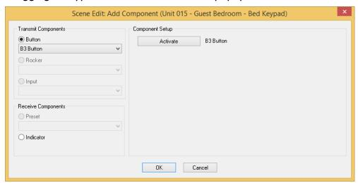
Like the wall switch, a keypad has both receive and transmit components. The buttons are transmit components and the LED indicators are receive components. After you choose which you want, press on the button in the Component Setup box and you can change what the button does:
