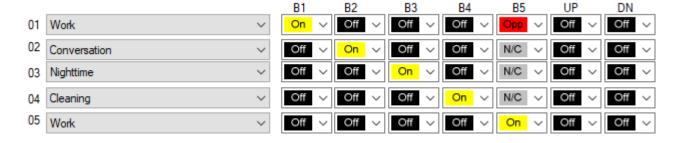
The Add Wizard for the KPLD-7 lets you pick the general operation of the keypad. When you do that UPStart pre-configures the indicators. After you add the scenes for the buttons, the "Indicators" tab has a method to copy those scene names over into the indicators.
