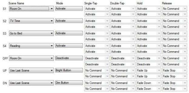
Note that none of the buttons toggle they all just activate scenes. Each button either activates a scene or, in the case of the OFF button, deactivates the scene. This is the configuration of the indicators:
