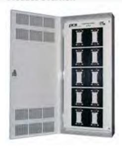
The Lighting Control Panel will simplify the design and installation of large PulseWorx Lighting Control Systems. The LCP-U panel will house up to twenty WS1DL-6 dimmers, or fifteen WS1DL-15 or ten WS1D-24L Dimmers controlling up to 20 individual circuits and delivering up to 24,000W of power. This is ideal for new construction or major remodel applications.
