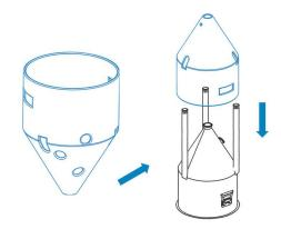
With the conical upside down and none of the accessories attached to the conical, slide the insulated jacket over the legs, welded ports and handles through all of the correlating holes.
