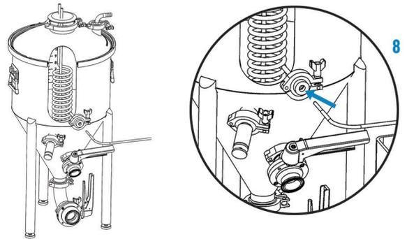
**8** Push the temp probe from the controller all the way into the thermowell port
