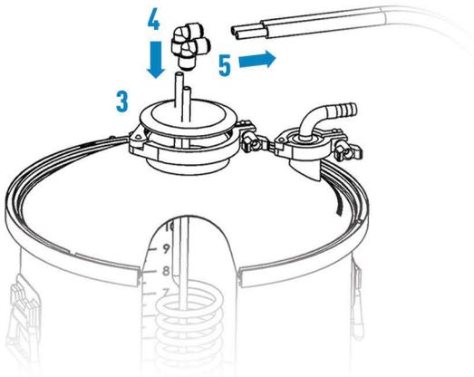
**3** Flip the conical right side up, attach your lid to the conical, and affix your temp coil to the 4" TC port
