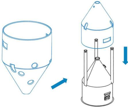
**2** With the conical upside down and none of the accessories attached to the conical, slide the insulated jacket over the legs, welded ports and handles through all of the correlating holes.
