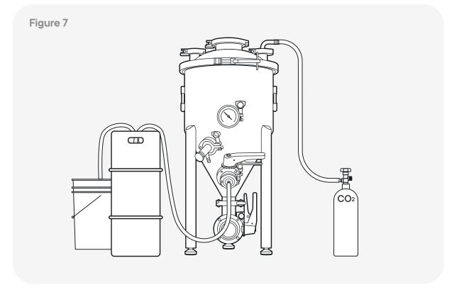
**PRO TIP:** If you are using a racking arm, we recommend starting your transfer with the racking arm in the up position and you can slowly rotate the racking arm down until the wort no longer runs clear. The position of the racking arm can be determined by using the indicating post welded to it. To turn the racking arm, loosen the clamp that attaches it to the conical by about 1 turn. Using the valve handle as leverage, you'll be able to slowly turn the racking arm to the desired position.
