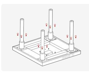
**3.** Slide the table support bracket over the 4 table legs and secure to each leg using 1 screw and 1 lock washer per leg.
