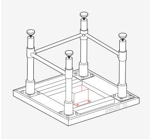
6. Flip the table over so that it is resting right side up. Gently place the mill onto the table and then use 4XM6 screws along with 4 lock washers through the table to attach the mill.
