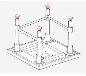
**5.** Slide the grain chute over the welded studs on the bottom of the table and secure with 4 nuts.
