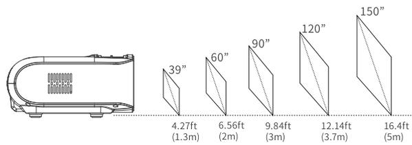
The recommended projection screen is around 80 inches with a projection distance of around 8.5 ft. Ambient darkness will improve the clarity of the projected images.
