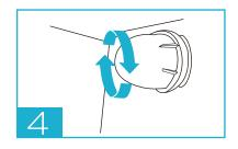
4.Rotate the light cover clockwise to tighten it.
