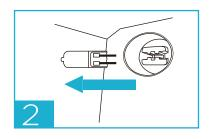
2.Remove the used bulb by pulling it directly.
