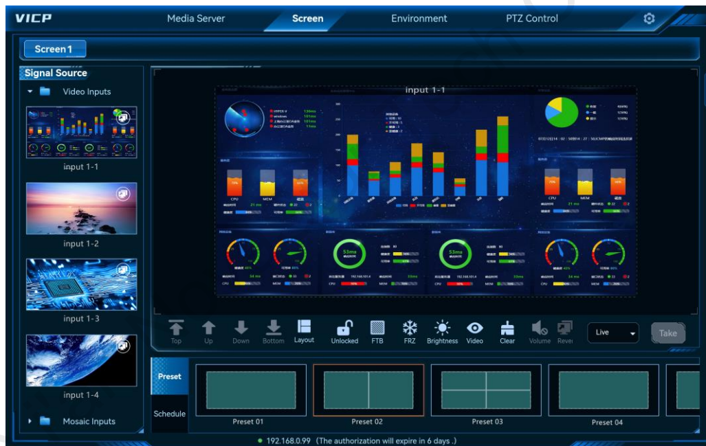
Figure 5-5 Input source switched successfully
