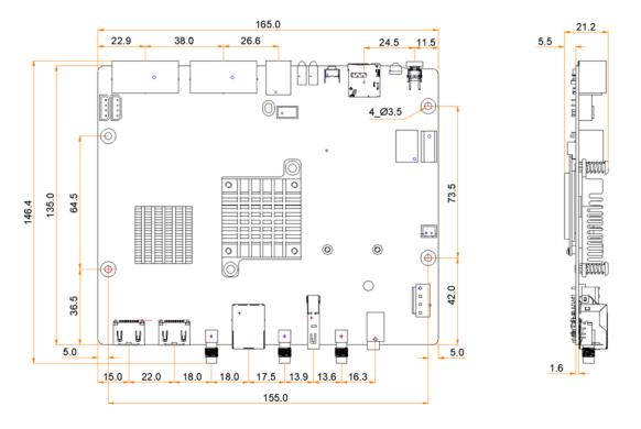
Tolerance: ±0.3 Unit: mm
