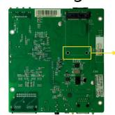
Without welded copper cylinders on the back
