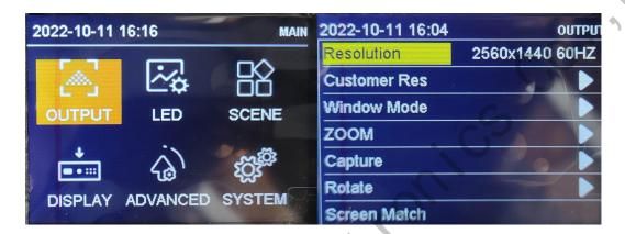
The system is preset with 18 types of output resolutions, When applied to the LED display, can choose a preset output resolution ,which is larger than that of LED screen resolution, or can customize set the output resolution according to the LED display.
