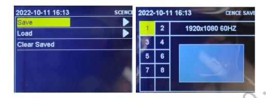
Here, can save and load the parameters set by the video processor, including input signal, input resolution, output resolution, position offset, scaling, interception and other information to save as templates for next time, the system has 8 templates for users to save.
