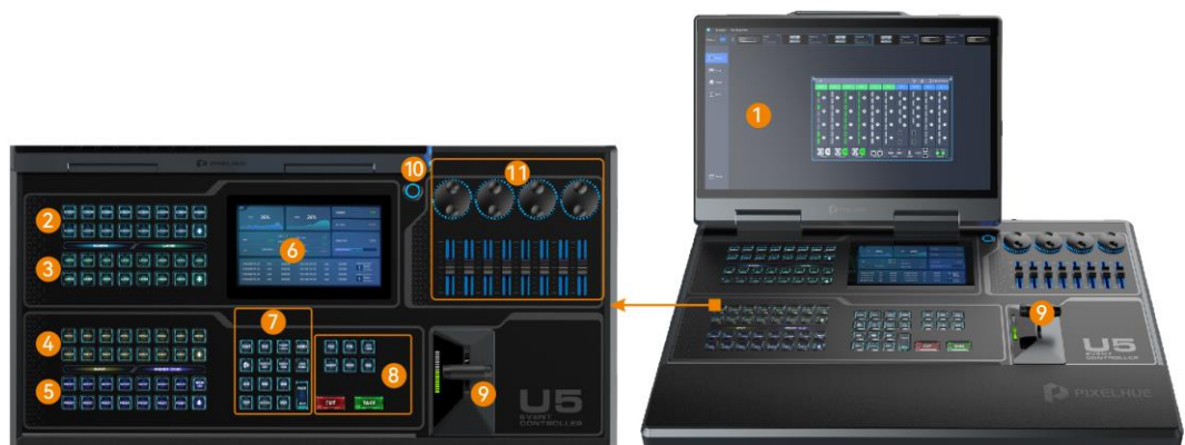
Figure 8-1 U5 front panel
