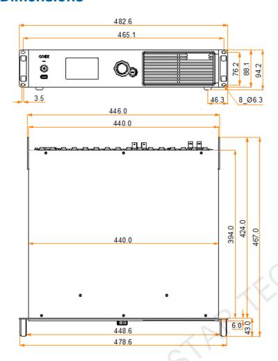
Tolerance: ±0.3 Unit: mm
