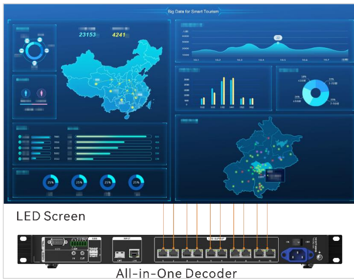
Figure 2-8 LED screen connections
