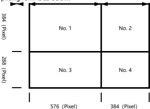
In this case there are four groups LED display screens, each group need a LED-550D. The four machines unequal splicing parameters must be set as the following table:
