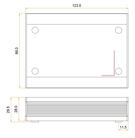
Tolerance: ±0.3 Unit: mm
