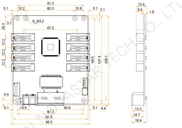
Tolerance: ±0.3 Unit: mm
