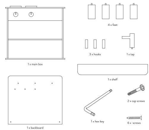
1 - Screw the tap on the countertop and the feet to the bottom.
