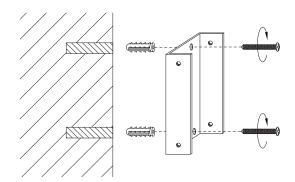
Set up the wall mount with two wall screws and two rawplugs.
