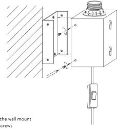
Mount the lamp on the wall mount and screw in 4 wall screws
