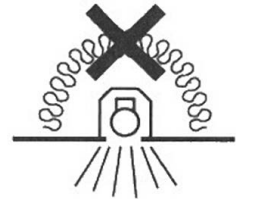
Luminaires not suitable for covering with thermally insulating material.
