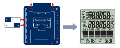
NOTE: When the batteries in the Energy Monitor are low on power, an indicator sign will be shown. Replace your batteries as described earlier.
