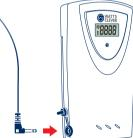
IMPORTANT: DO NOT connect the LED sensor until the pairing is done and the LED sensor is attached to the meter. This will stop inaccurate readings occurring from the LED sensor detecting normal light and indoor lighting.
