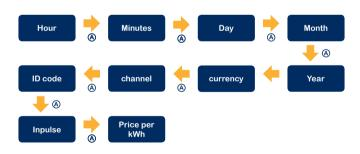
(A) Setup with ( and ( button. Press [ Select ( ) to confirm the value.
