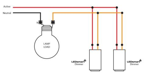
Two-way dimming and switching using LEDsmart<sup>+</sup> dimmers. Note the two-wire dimmers are simply wired in parallel.
