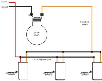
Rocker switches and intermediate switch replaced with LEDsmart<sup>+</sup> dimmers. The existing strappers are used to connect the dimmers in parallel. No new wiring is required.
