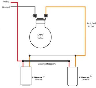
Rocker switches replaced with LEDsmart+ dimmers using the existing strapper wires. No new wiring required.
