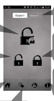
Press to change controls from relay 1 to relay 2 (useful for pedestrian gates)
