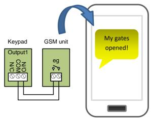
When the egress is triggered, the GSM unit's output 1 will be triggered and if the 78 feature is programmed, the unit will send an SMS.
