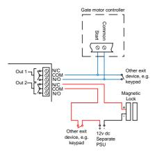
This example shows relay 2 connected to a gate motor controller for vehicle gates, and output 1 connected to a magnetic lock for a door or pedestrian gate.
