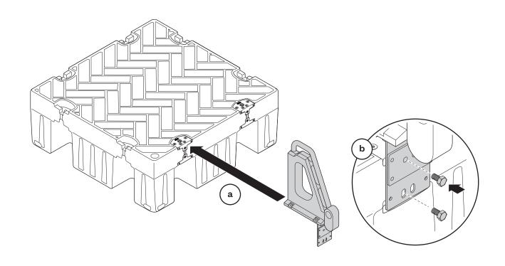
Place the second Ladder Bracket in place but do not attach it. Once the Ladder Brackets are in place, align Rungs with Ladder Brackets (a) and fasten the Rungs to the Ladder Handles with the provided hardware, two (2) 5/16" x 5" Partially Threaded Bolts, Washers and Lock Nuts (b). Fasten the second Ladder Bracket to the Flat Face Connectors using the two (2) 1/2"-13 x 3/4" Hex Head screws as performed in step (c).
