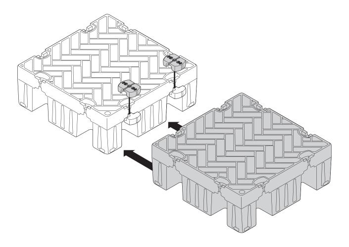
**Note:** Floats must be connected together to a flat face. You will not be able to attach the connectors to two sides of the float at once.
