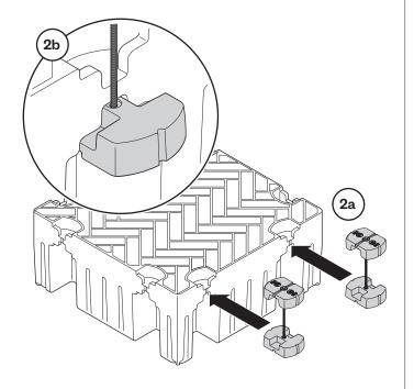
With the additional Float put into place, tighten each Bolt. Continue this process to arrange the remaining Floats.
