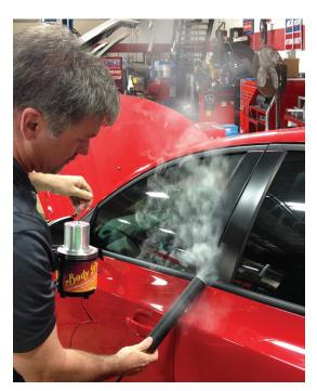
Improve Accuracy of Repairs Eliminate comebacks by verifying that leaks are repaired completely.
