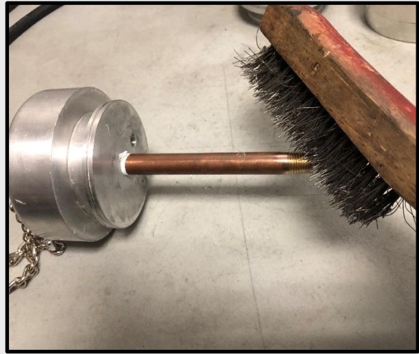
Clean threads on pipe nipple with wire brush.
