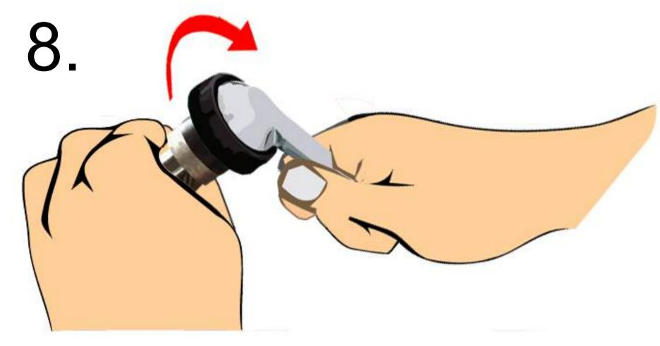
Hold blade firmly in one hand and turn handle clockwise. (Be careful as the blade is very sharp.)
