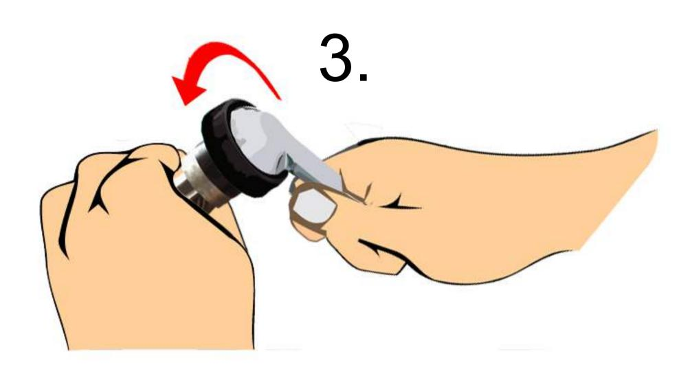
Hold blade firmly in one hand and turn handle counterclockwise. (Be careful as the blade is very sharp.)
