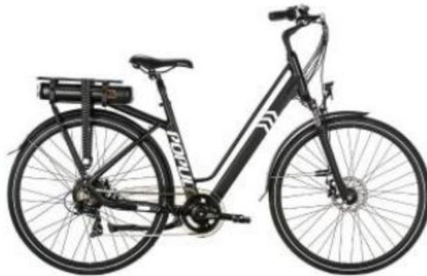
The step through e-bike is all to do with the design of the frame of the e-bike. It eliminates the upper crossbar.
