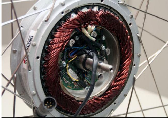
Geared HUB: These contain planetary gears and are smaller, lighter, and provide more torque and less drag when pedaled. On the other hand, they are less durable, noisier, and have a lower top speed. They are best for steep hills and heavy loads.
