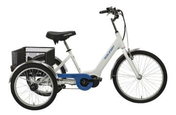
The three wheels of the trike bring obvious stability to the biking experience with battery power providing a pedaling boost. The riding position is upright or recumbent.
