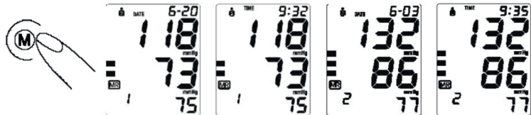
(MR1: Values of the last measurement) (MR2-MR60: Values of the measurement before MR1)
