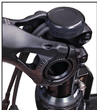
Example: A-Headset assembly (optional)
