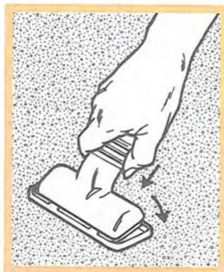
ATTACHING THE SUCTION RELIEF UPHOLSTERY PANEL
