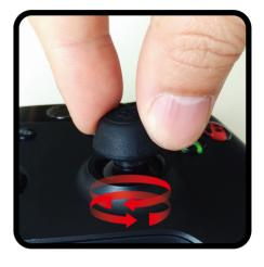
**Step 3**Rotate the grip until the edge wrap up the joystick.
