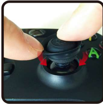
Step 2 Put the grip on the joystick, fall the edge of the grip.
