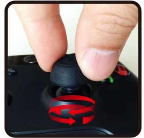
Step 3 Rotate the grip until the edge wrap up the joystick.
