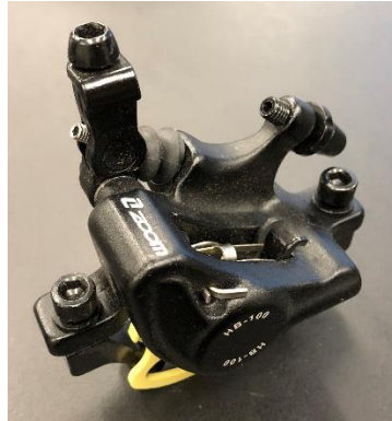
Rear Brake Pad Set with Retaining Spring and Cotter Pin
