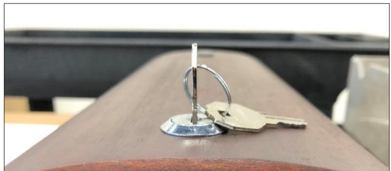
Battery Cover Lock – Installed
