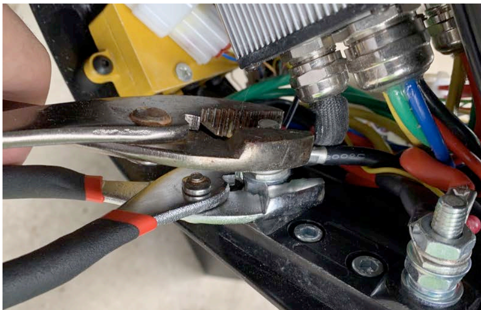
Figure 13: Loosening Ground Lug Nuts for Spade Connection
