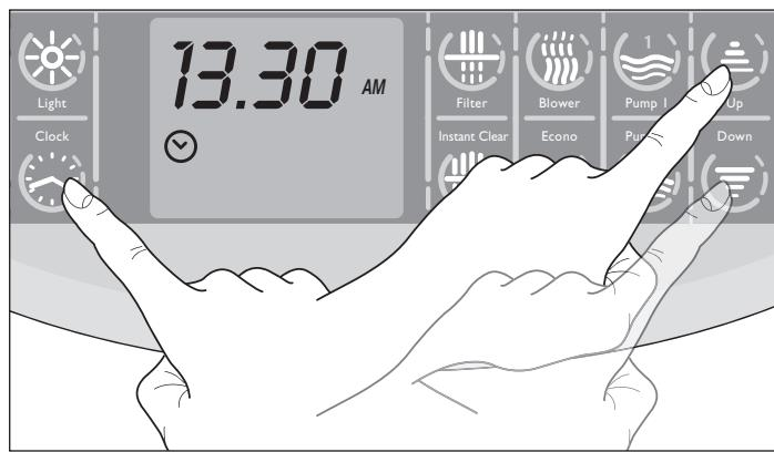
► Press the “Clock”
