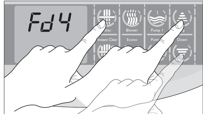
► Press the key “Filter”
