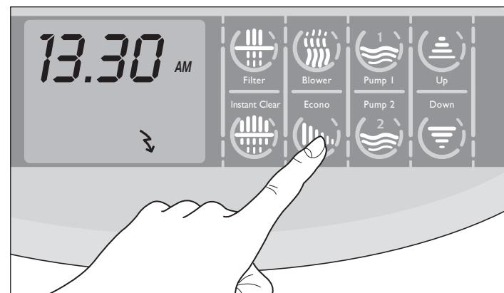
► Press the key "Econo" . The display shows the message **Edx**, where "x" indicates the duration in hours.
